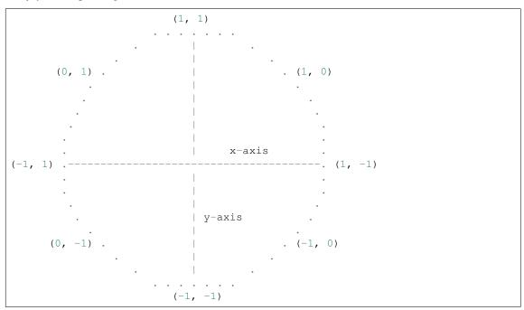
The joystick is a circle within a circle where the (x, y) coordinates of the joystick form an angle with the x-axis. Our job is to translate this angle into the percentage of power that should be sent to each motor. For instance if the joystick is moved all the way to the top of the circle we want both motors to move forward with 100% power...that is represented above by (1, 1). If the joystick is moved all the way to the right
